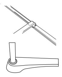
3. Unsnap the lock of adjustable pole and fit the endtip of the adjustable pole to the slot of the top profile.
