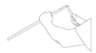
2. Lock the foot onto the slot of the bottom profile.
