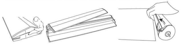
With our V4 Dual Roller, there are two choices for you to attach your graphics to the roller. If you wish to attach the graphic to its snap side, open the snap roller, then insert your graphic onto the roller. Press hard onto the centre of the roller, to ensure it is shut tightly. Then, press hard on the ends of the roller, to ensure it is completely tight and shut.
