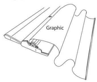
6. Push the graphic slightly away from the base to activate the spring mechanism. Whilst holding onto the graphic, remove the locking pin and allow the graphic to gently retract into the base.
