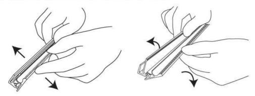
2. Feed the graphic into the gap in the center of the roll back rail, then press hard along the entire rail to close it tight.
