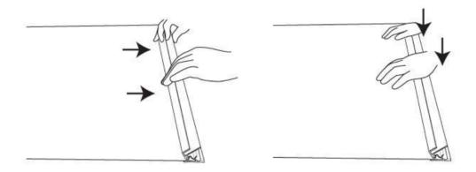
3. Click the buttons on both end caps to totally remove the cover. Remove the roller mechanism from the base and gently open the snap rail on the roller by hand.
