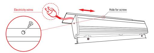
Please fix with screw in centre after pushing the body in frame to right side or left side.
