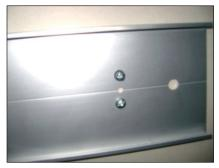
Fix mounting bracket using appropriate fixings (must suit bearing weight of 18kg or more). Where possible fix to timber or aluminium roof structure.
