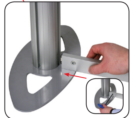
Attach top and bottom horizontal extrusions to the vertical uprights using the installed lock and the supplied hex key.
